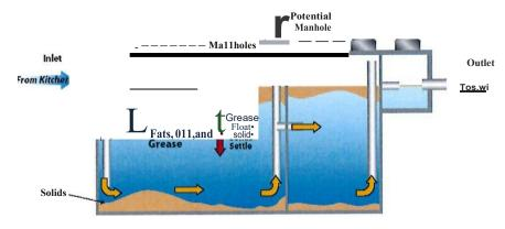
CONVENTIONAL GREASE INTERCEPTOR Outdoor, In-ground-Precast Concrete (Typical)
